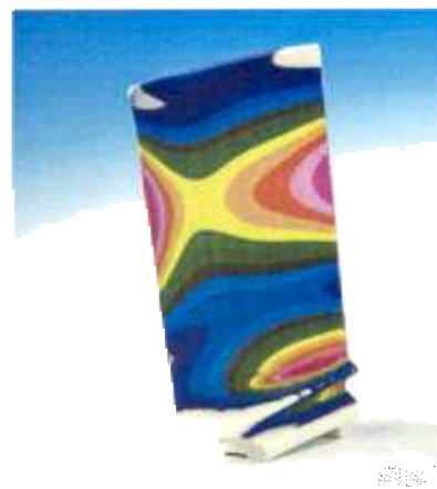
Turbine blade showing FEA output.
